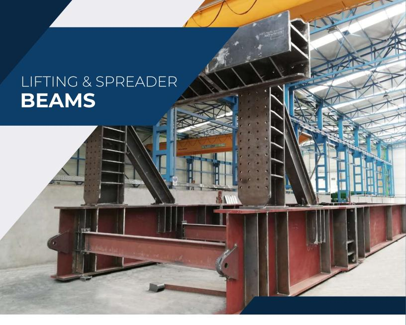
Besides our main products, we produce heavy lifting and spreader beams and uprighting frames for industrial services. These beams are designed and manufactured as per international standards, tested up to 700-ton loading with our special loading machine in our workshop. All beams are offered with CE certificates.
